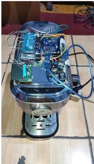
Gambar 3 Prototype mesin Kontrol espresso
